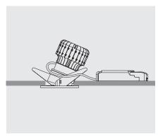
4. Adjust the angle required. Installation complete.
