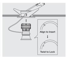
3. Gently insert module holder from the bottom of the fixture frame.
