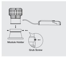
2. Grub screw to tighten between module & module holder and connect module to driver.
